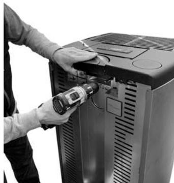
Fig. 78 - Retirer le bouchon (Atena³ Plus 12/14 - Duke At)
